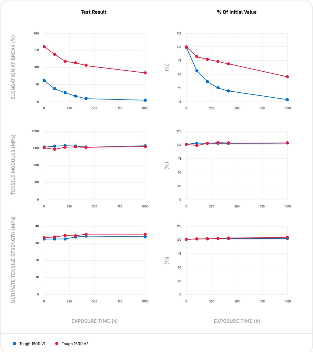
ASTM D4329: Cycle A for general applications, QUV/iso, UVA 340 nm, 0.89 W/m<sup>2</sup>-nm, 8 hours UV light at 60°C followed by 4 hours at 50°C condensation in the dark. To reduce any sample warpage during test time samples were placed in tailor-made holders without any fixation clamps or mechanical load. Exposed samples were always removed from QUV before next condensation cycle to avoid samples that are soaked excessively with water before testing.
